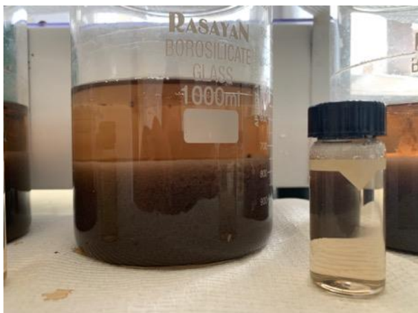
Figure 1. Turbidity removal and treated DAF effluent.
